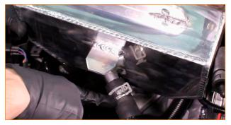
13. Compress the spring-clamp that secures the coolant hose to the rear of the expansion tank, and slide it down the hose. Then disconnect the hose from the expansion tank, and remove the tank from the vehicle. (1x spring-clamp) 14. Compress the spring-clamp that secures the upper radiator hose to the vehicle, and move it down the hose. Then disconnect the hose from the radiator. (1x spring-clamp)
