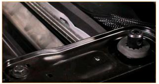
Remove the two bolts that secure the passenger-side radiator stay to the vehicle, and then remove the radiator stay. (2x 10mm bolts)
