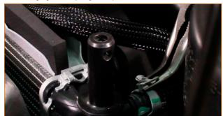
Remove the two bolts that secure the expansion tank to the fan shroud. (2x 10mm bolts)
