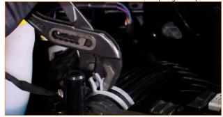
Disconnect the fan wiring harness. Depress the lock tab on the connector, then slide the connector apart.
