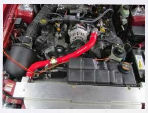
**Figure 2**: PLX sensors were attached to the vehicle to obtain inlet and outlet temperatures from the radiator
