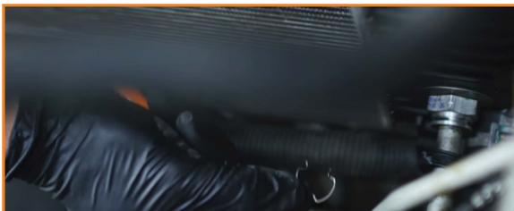
12. Remove the bolts on the upper radiator brackets. (2x 13mm bolts)
