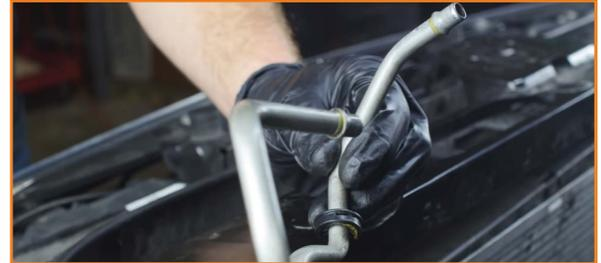
14. Drain your coolant system. This requires disconnecting the lower hose on the reservoir tank. (1x spring clamp)
