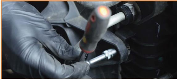
9. Separate the upper oil cooler line from the radiator. Slide the clip cover down the line, and then pull out the clip that secures the connection. Plug the line to prevent spillage. (1x spring clip)
