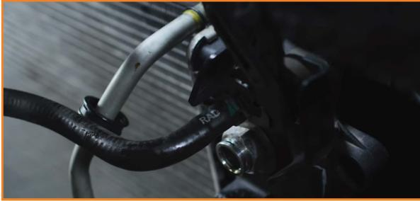
17. Remove the bolt that holds on the AC condenser lines, which is located on the passenger side of the radiator end tank. (1x 10mm bolt)
