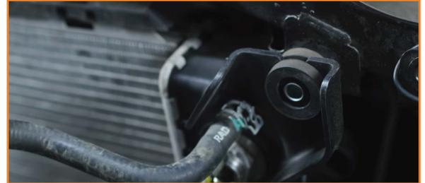
13. Remove the transmission cooler line from the radiator. (2x spring clips)
