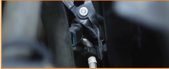
8. Remove the bolts that secure the fan shroud to the radiator. (2x 10mm bolts)
