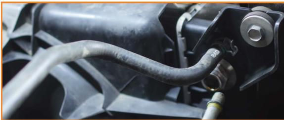
10. Lift the fan shroud out of the engine bay.
