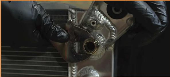
22. Lower the Mishimoto radiator in at an angle. Then secure the AC condenser line located on the passenger side end tank. (1x 10mm bolt)
