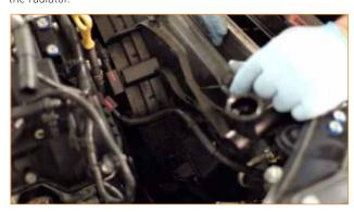
11. If your vehicle is equipped with an automatic transmission, disconnect the lines at the base of the radiator. An external transmission cooler will be necessary if installing this on an automatic model.
