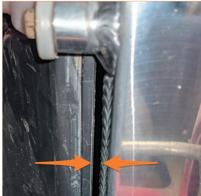
**03.** Install Mishimoto radiator the same way you would install a stock radiator, using original hardware.
