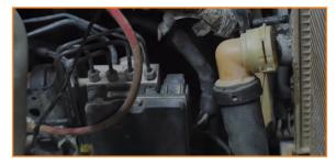
14. Compress the clamp on the overflow hose and slide the clamp down the hose. Then slide the overflow hose off the radiator. (1x spring clamp)
