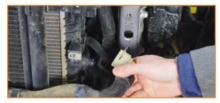
17. Remove the two bolts that secure the AC condenser. (2x 10mm bolts)
