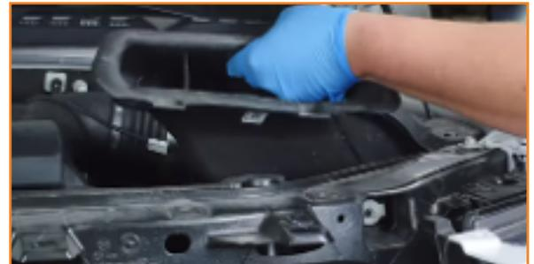
3. Remove the clips from the corner panels along each side of the grille. The clips are located at the top of the panels. (2x pop-clips)
