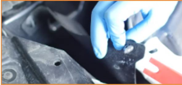
7. Disconnect the grille shutter, camera, and washer fluid harnesses. Separate the wiring from the clips that secure them in place. (2x tree clips)
