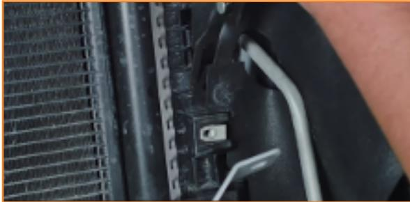
14. Compress the clamp on the overflow hose and reposition the clamp down the hose so it clears the barb. Slide the hose off the radiator port. (1x spring clamp)
