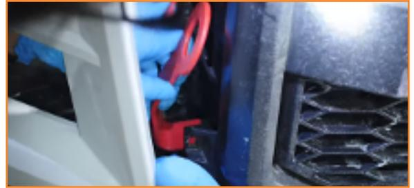
11. Free the bracket that holds the transmission line on the driver side. (1x 10mm bolt)
