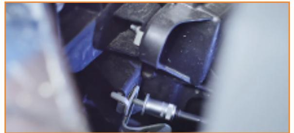
19. Disconnect the two fan harnesses and release the clips holding the harness to the fan shroud. (11x tree clips)
