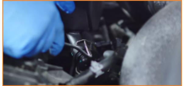
18. Unscrew the bolt on the bracket that holds the driver-side transmission line. (1x 10mm bolt)
