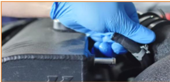
16. Remove the bolts that secure the expansion tank. (2x 10mm bolts)
