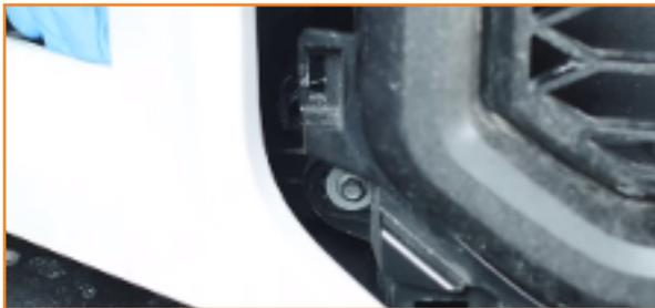
9. Release the clips on each side of the grille. You will need to lift the grille to reach these clips. Lift the grille off the vehicle once free. (2x tree clips)
