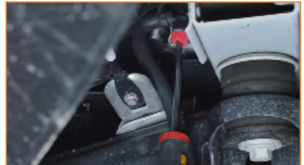
2. Remove the intake duct.
