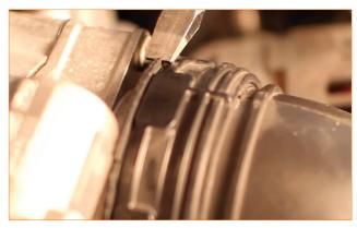
19. Position an oil drain pan beneath the radiator, where the transmission lines are attached. Remove both transmission lines by pulling back the dust boot and using a pick or similar tool to remove the E-clips from the fitting. The clips are quite small and easy to lose, so be very careful here. Once the clips are removed, the lines can be pulled out of the fittings. [2x E-clips]
