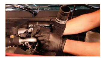
10. Remove the coolant overflow hose from the radiator, and tuck it out of the way.
