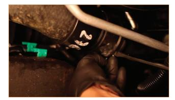
09. Remove the upper radiator hose by squeezing the clamp and sliding it up the hose. Then slide the hose off the radiator inlet. Tuck the hose back and tie it out of the way. This hose should be empty, but there may be some residual coolant.
