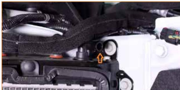
24. Compress the clamp that secures the outer hose to the radiator and slide the clamp down the hose. Remove the outer hose from the radiator. (1x spring-clamp)
