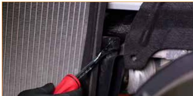
26. Remove the brake cooling duct from the vehicle.
