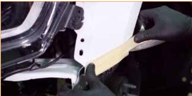
**59.** Install the front bumper. Align the pins on the bumper with the holes in the fender as you slide the bumper over the nose of the vehicle. Lift the top edge of the bumper over the alignment tabs. Check the fender gap on both sides, and then remove the masking tape.
