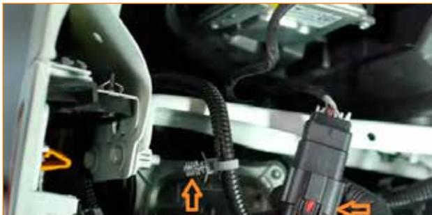
16. Remove the seven screws and one pop-clip that secure the passenger-side fender liner to the vehicle. (7x T15 screws, 1x pop-clip)
