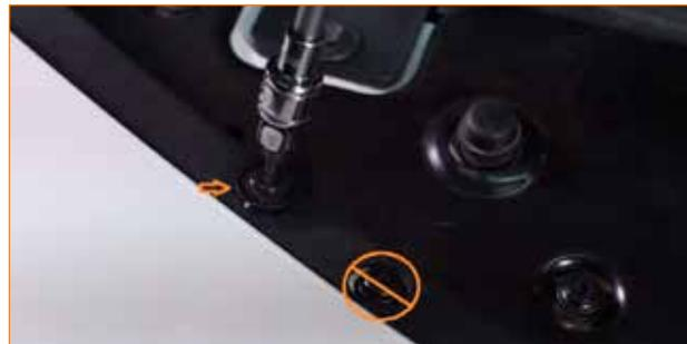
03. Remove the five screws that secure the air diverter to the driverside of the vehicle and remove the air diverter. Repeat this process on the passengerside. (10x 7mm screws)
