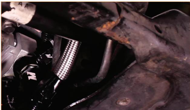
32. Mark the free end of the hose attached to the **OUT** port with painters tape to identify it later.
