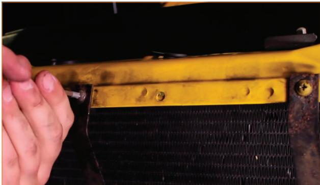
15. Gently pull the power steering cooler forward, and remove the passenger-side cooler support bracket.
