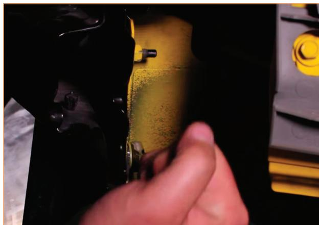
11. Remove the two pop-clips that secure the air diverter to the crash beam. (2x pop-clips)
