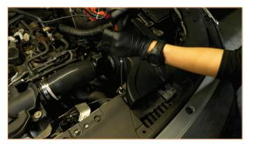
**12.** Clip the MAF harness to the Mishimoto airbox, then reconnect the sensor.
