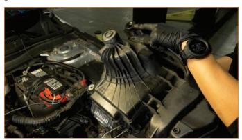
**6.** Transfer the MAF sensor from the stock airbox to Mishimoto MAF housing, install with provided hardware. (2x 2.5mm button head bolts)
