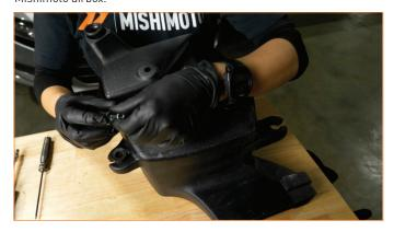
8. Assemble the rubber grommet, MAF housing, and air filter as shown.
