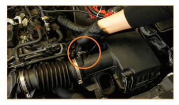
4. Remove 2x 10mm bolts securing the stock airbox.
