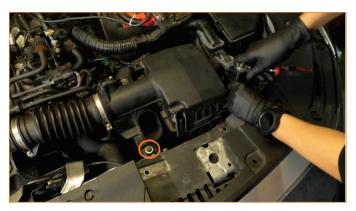
**5.** Remove airbox from the engine bay. Make sure the bottom rubber grommet comes out with the airbox.
