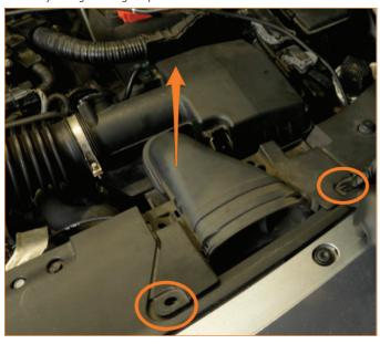
2. Unclip the MAF sensor harness from the airbox.
