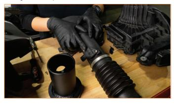
**7.** Transfer the 3x mounting grommets from the stock airbox to the Mishimoto airbox.
