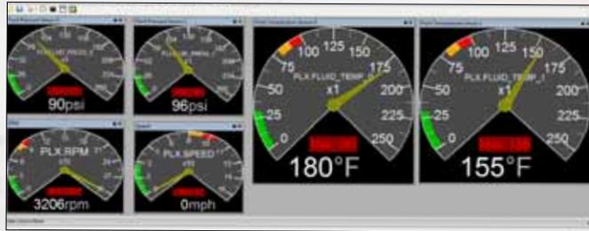
Fluid temperatures were taken from both the inlet and outlet of the 25-row oil cooler, using custom inline sensor housings and PLX fluid temperature sensors. Oil pressure was also tested to ensure no dramatic pressure drop occurs when installing the oil cooler.
